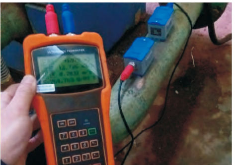
Ultrasonic flow meter for clean water measurement
